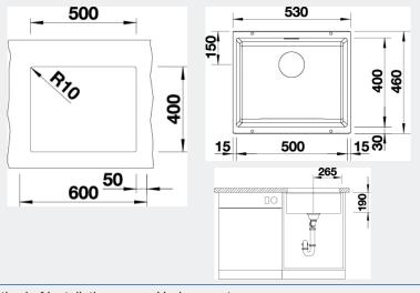
Undermount Method of Installation:
