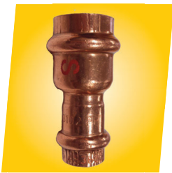
Ezi Press™ Solar fittings are manufactured in high quality copper and/or DZR brass material with a factory-fitted high performance red (FKM) sealing element.
